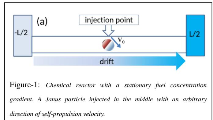
Figure-1: Chemical reactor with a stationary fuel concentration gradient. A Janus particle injected in the middle with an arbitrary direction of self-propulsion velocity.
