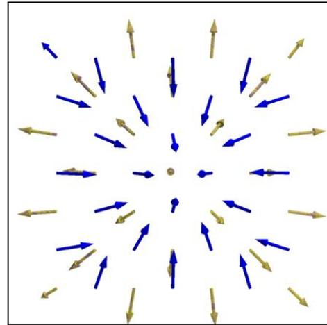
**Figure 2: antiferromagnetic skyrmion**
