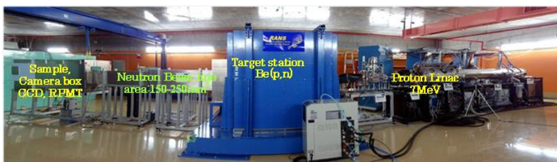
Fig. 1 Panoramagram of RANS (center: target station; right: proton Linac accelerator; left: beam dump)
