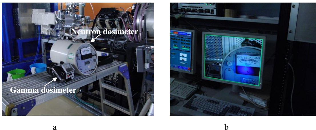
Fig. 8 Scene of measurement (a. Neutron and gamma radiation measurements by dosimeters; b. Reading radiation value from display at operating area by using web camera)
