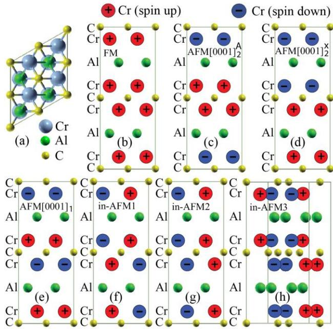
FIG. 2. Schematic representations of seven initial spin configurations considered for Cr<sub>2</sub>AlC MAX phase.
