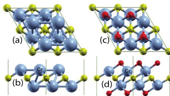
FIG. 1. The top views of 2x2 models of (a) the bare MXene  $Cr_2C$  and (c) the MXene  $Cr_2C$  functionalized by F group considered in this study. (b) and (d) show the side views of (a) and (c) structures, respectively.
